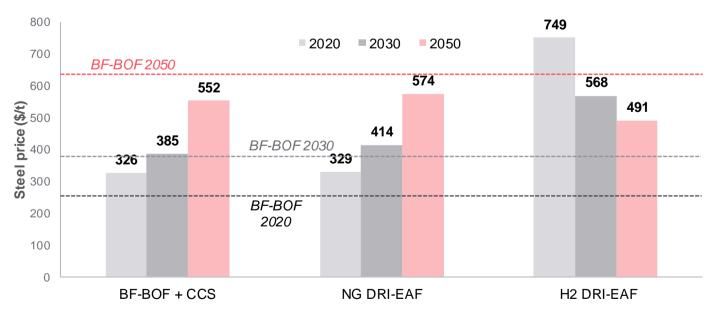
With steel prices increasing by 10% YoY till 2050, it is expected that the cost of steel manufacturing with the integration of CCS or using Natural Gas (NG) as feedstock will become cost-competitive as compared with traditional manufacturing techniques by 2030. While steel manufacturing using Hydrogen ( $H_2$ ) as feedstock could become cost-competitive by 2050
