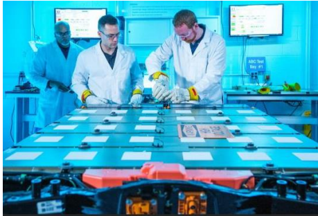
The wireless management system, developed with Analog Devices, Inc., helps balance chemistry within the individual cells.
