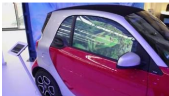
Gauzy's smart glass with liquid crystal and SPD technology
