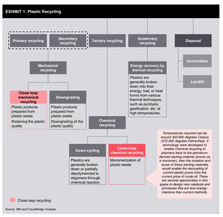
Key steps involved in the chemical recycling process include: plastic is chopped up and treated with the combination of water, heat, pressure, and enzymes or catalysts, breaking the resin down into its constituent parts. These chemicals are repolymerized into virgin-quality resins or used as fuel or as raw materials for other products. *(refer Table 1)*
